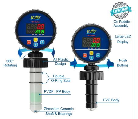
The TIP digital flow meters are easy to install with exceptional long life performance. Truflo TIP Series Paddle Wheel Flow Sensors are highly repeatable, rugged sensors that offer exceptional value with little or no maintenance. The TIP Series has a process-ready open collector signal with a wide dynamic flow range of 0.1 to 10 m/s (0.3 to 33 ft/s). The sensor measures liquid flow rates in full pipes and can be used in low pressure systems.
